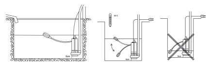
Never suspend the pump by its electric cord, if it is necessary that pump does not touch to the bottom, suspend it by a plastic cable fixed to the transport handle.
